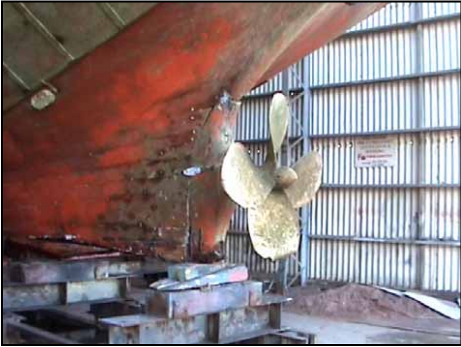
Photograph 4 Skag. The skag is completely missing from where it was scarfed into the keel. The holding bolts have been torn out.
