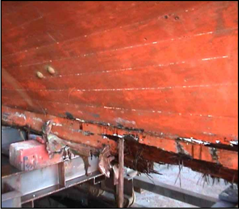
Photograph 3 Keel. The entire length of the keel has impact damage.
