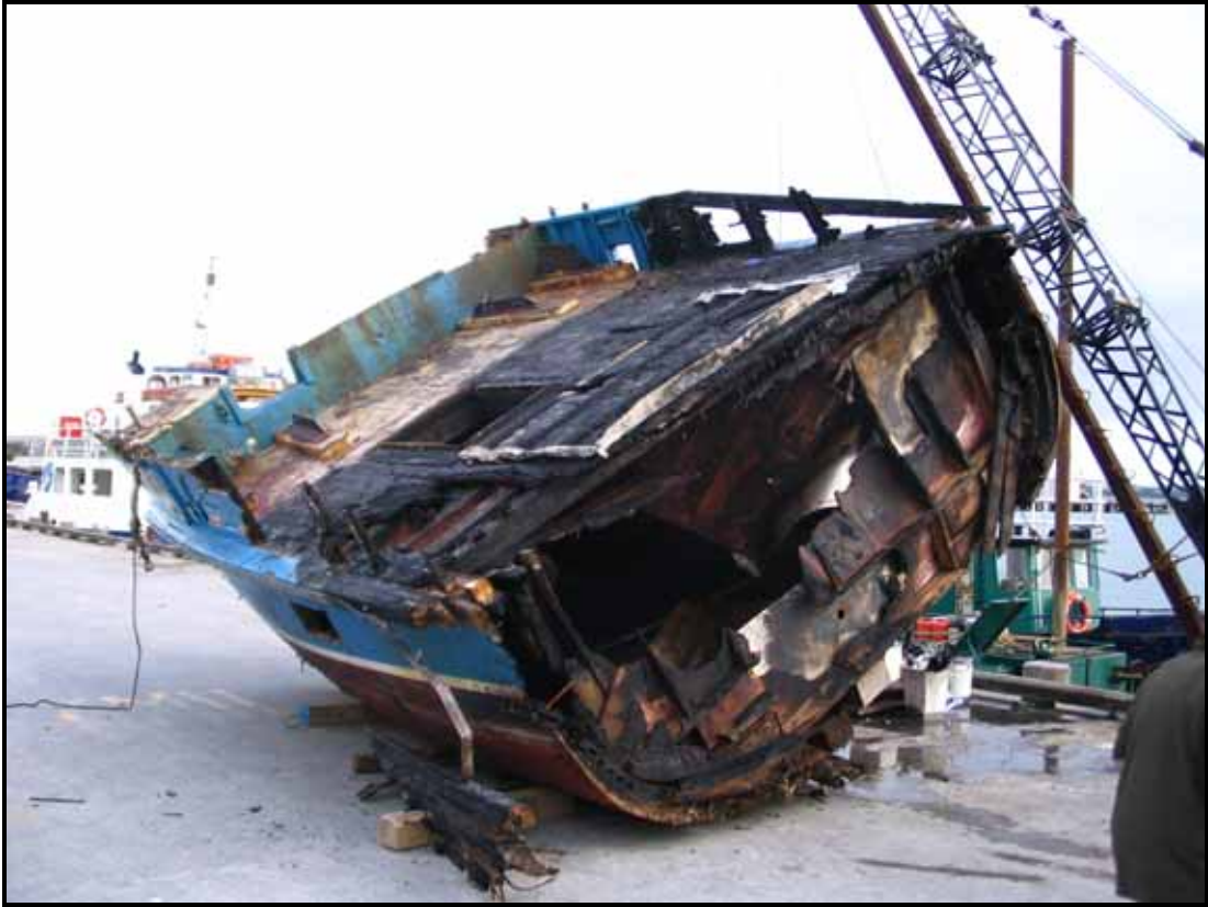
Photograph 3 Forward section of hull (fish hold) after salvage
