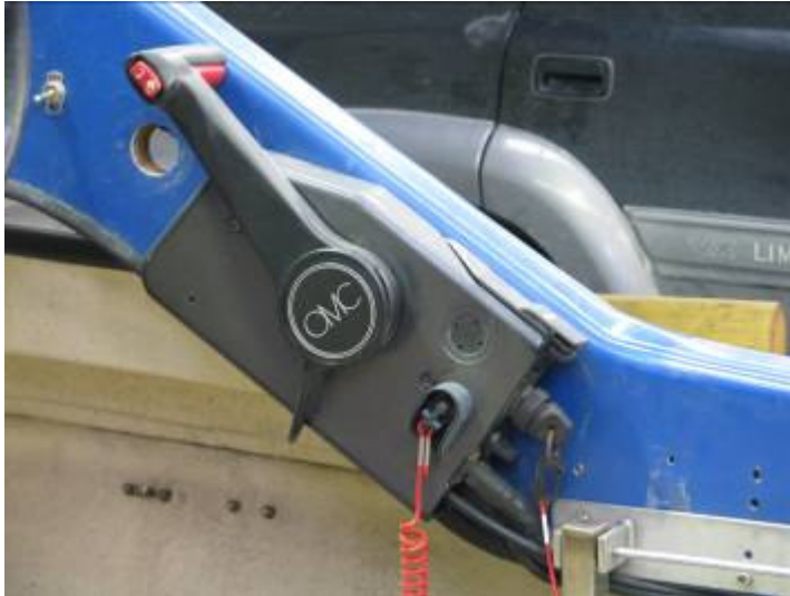
Figure 14 Throttle control, emergency stop switch and lanyard
