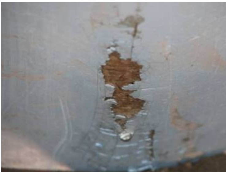
Figure 7 Impact damage on the keel
