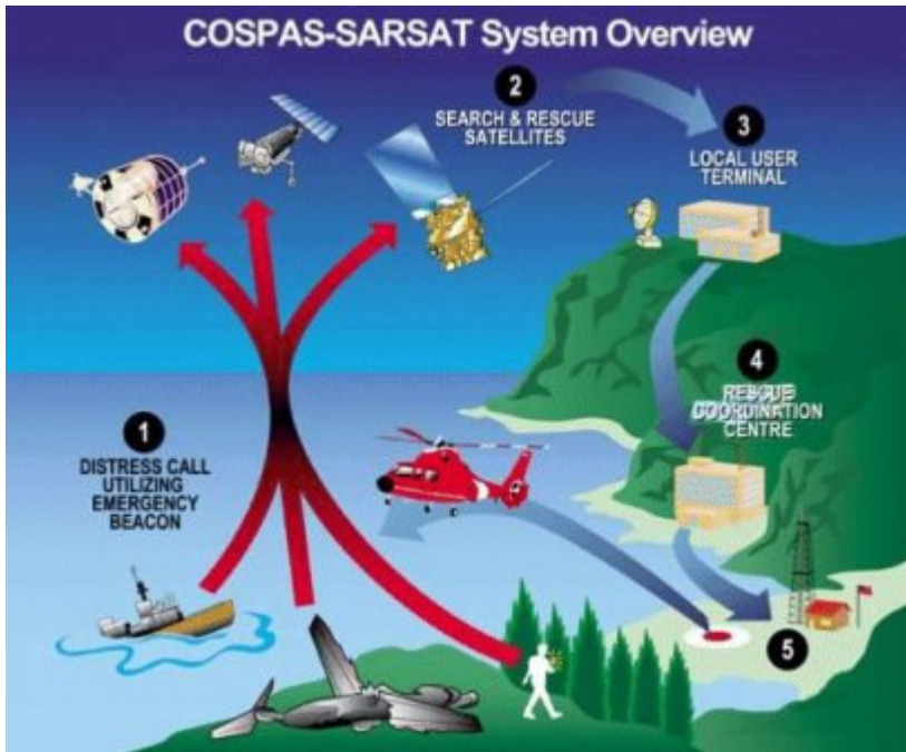
Figure A1.1 How the COSPAS-SARSAT system works
