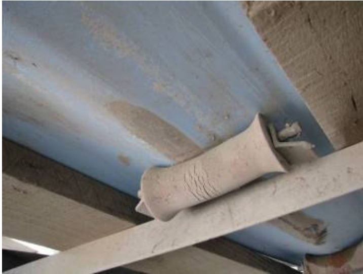
Figure 3 General wear on the keel
