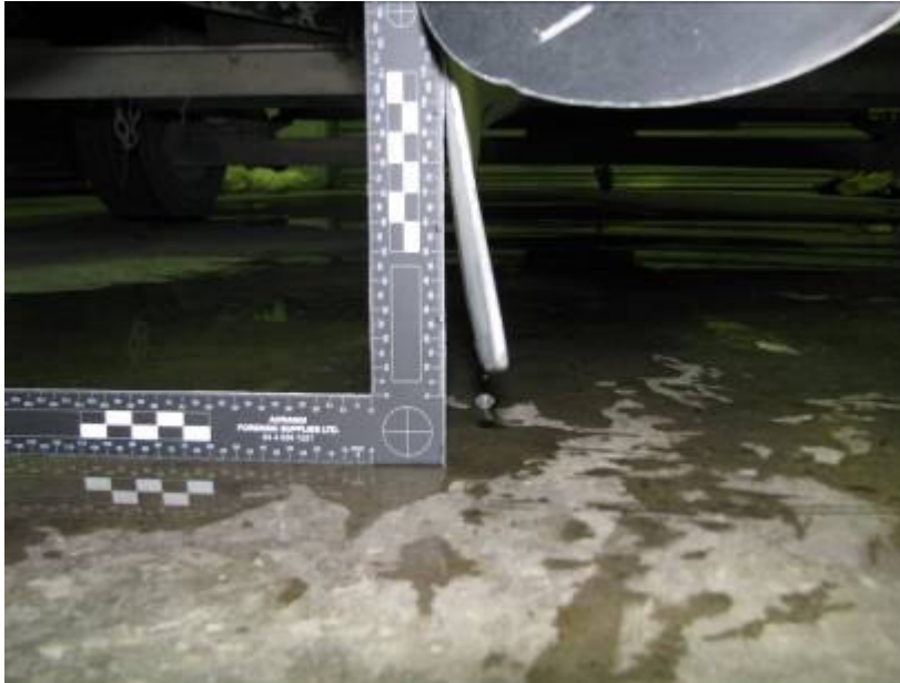
Figure 13 The bent skag
