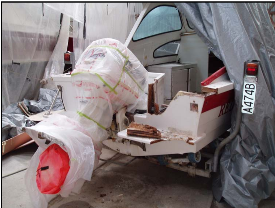
Photograph 3 Damage to the transom of Red Pepper
