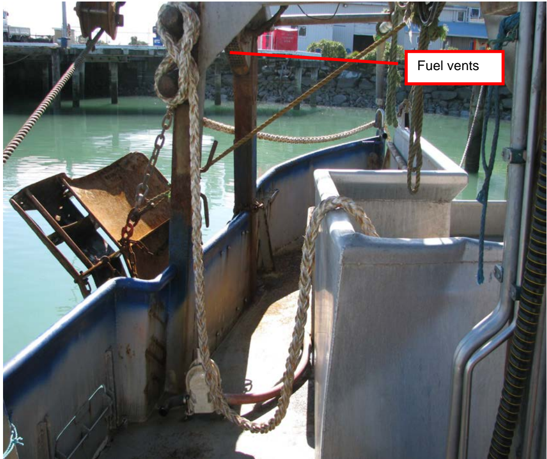
Figure 3 Fuel vent on the gantry
