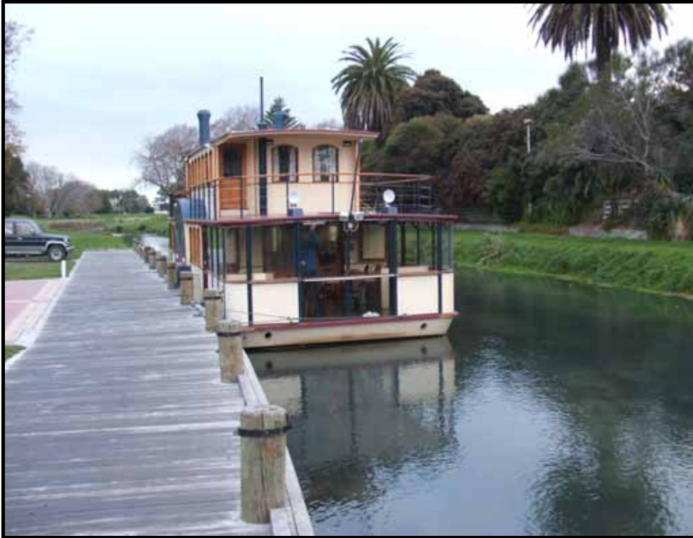
Figure 2 Vessel alongside berth, note two passive vent holes in the stern.
