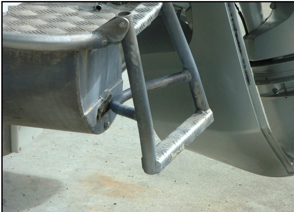
PHOTO 2 – DAMAGED BOARDING LADDER
