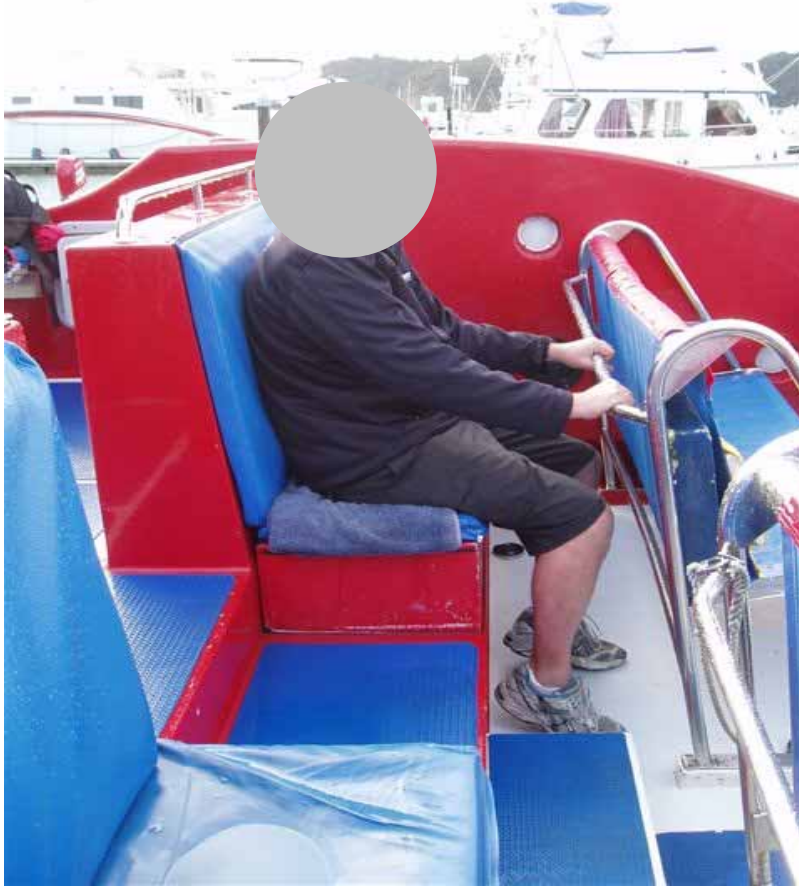
Figure 22 Alternative bench seat on Excitor showing that low forearm angle which allows for greater lumbar instability compared to a higher forearm angle
