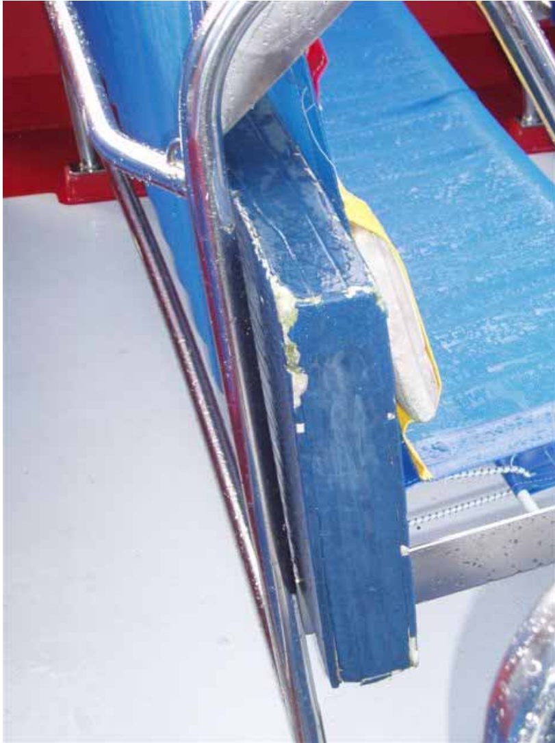
Figure 24 Showing wear on padding in its stored position.
