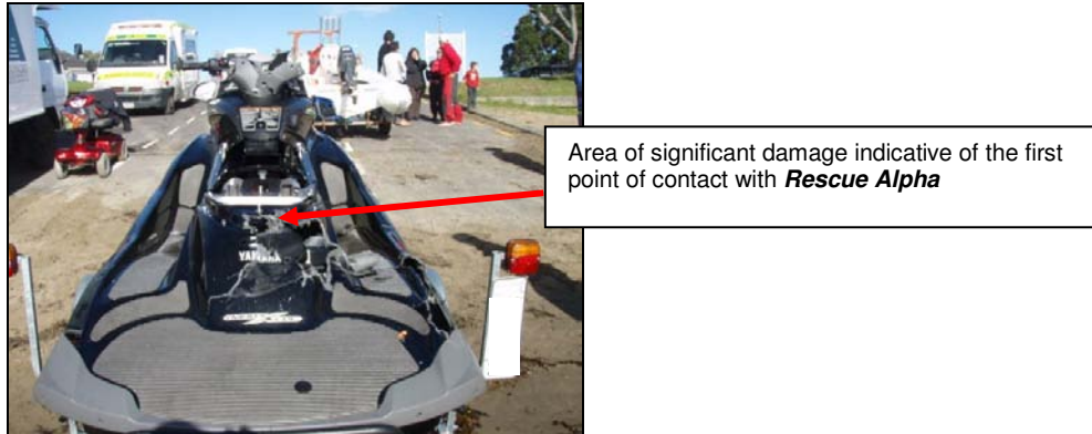
Figure 2 Photograph showing damage sustained by PWC 911
