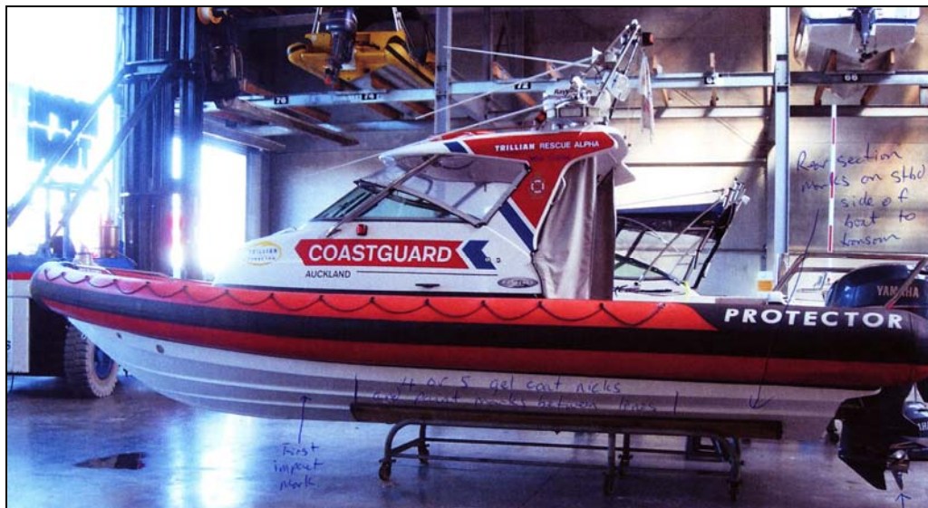
Figure 3 Photograph showing damage sustained by Rescue Alpha . Handwritten notes explaining areas of damage.
