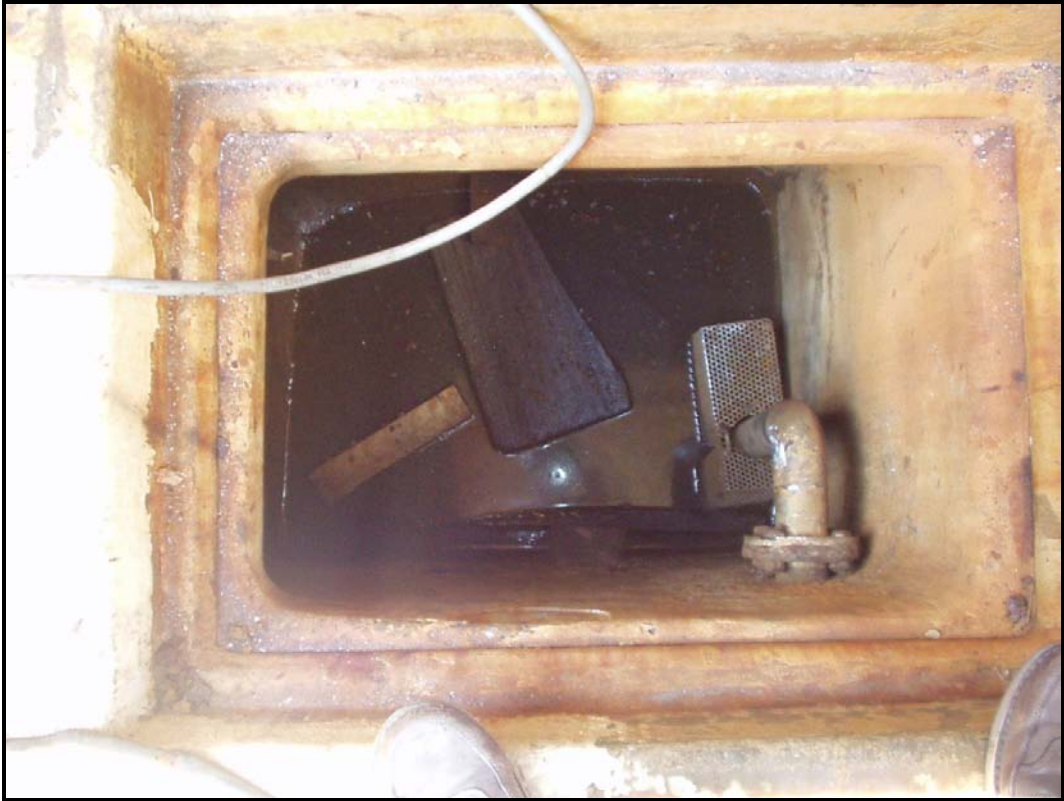
Photograph 2 Port Bilge Sump
