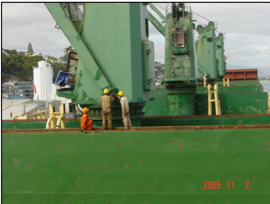
Photograph 10 Showing crew standing on hatch cover while working on No. 4 crane because there was no working platform fitted.
