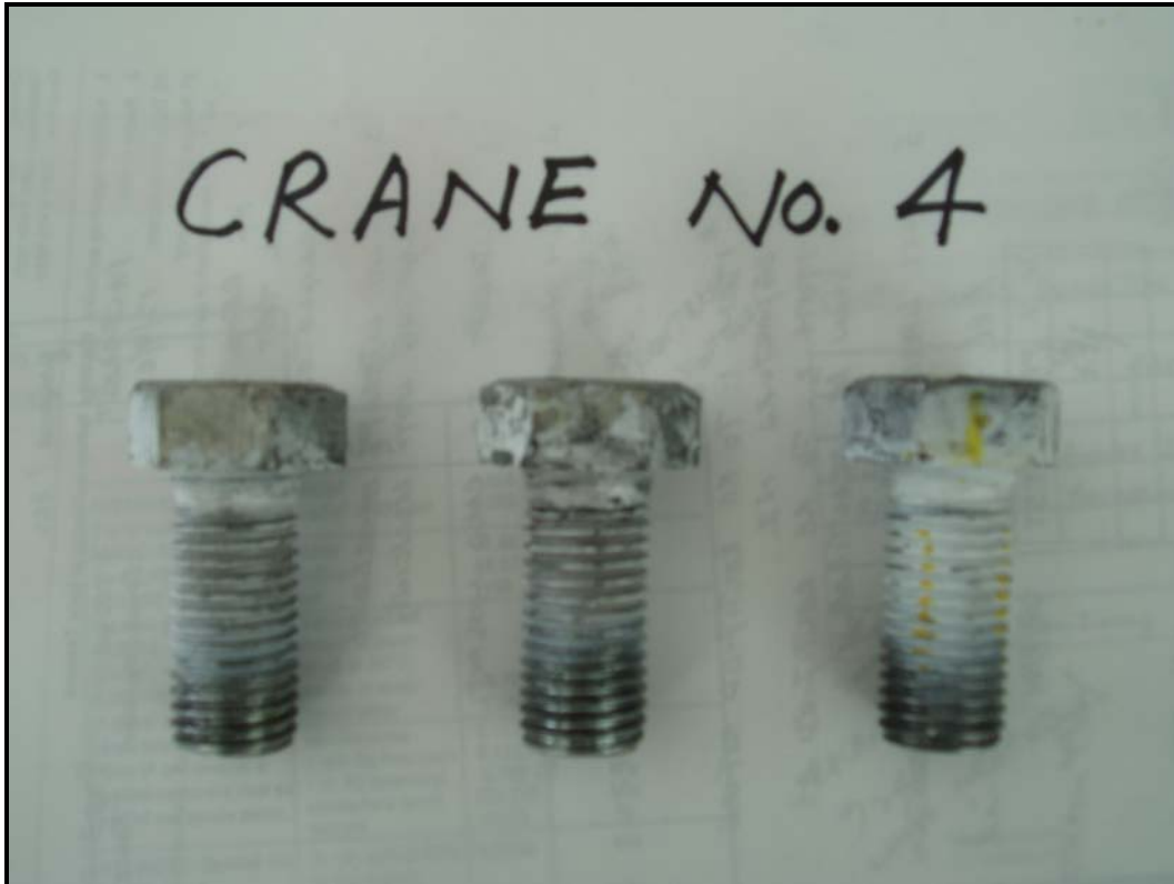
Photograph 9 No. 4 crane heel bolts indicating crack by Magnetic Particle Test
