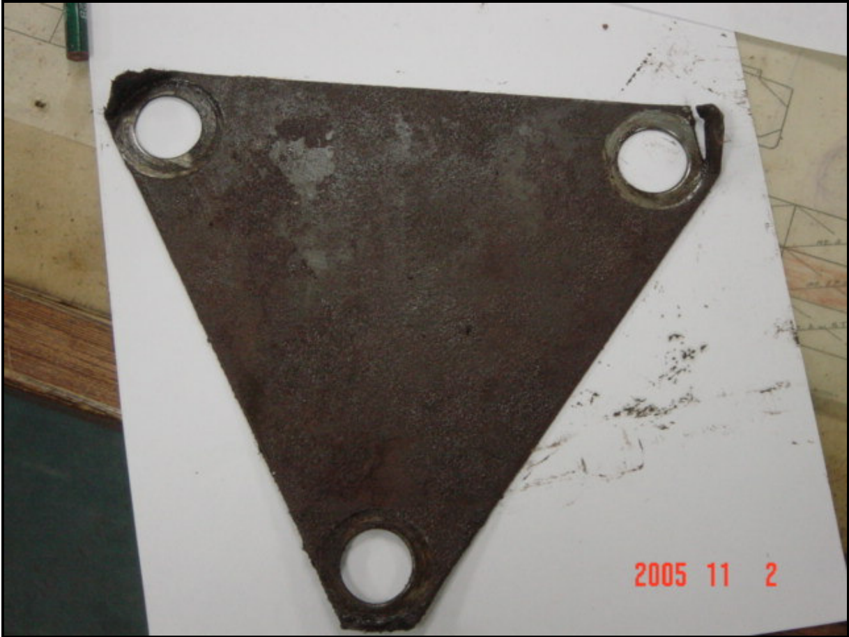
Photograph 11 No. 3 Crane heel bolts locking plate showing crack
