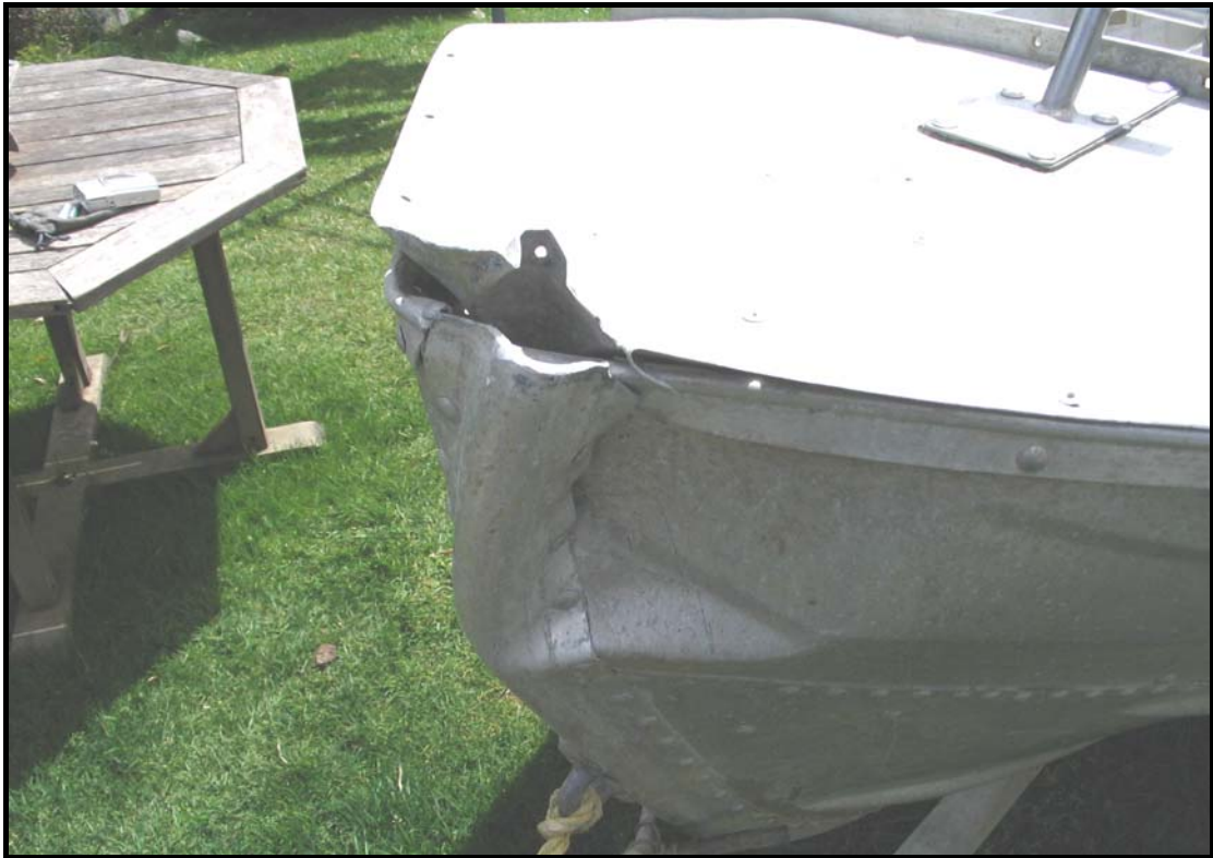
PHOTO 1 – DAMAGE TO BOW OF UNNAMED DINGHY
