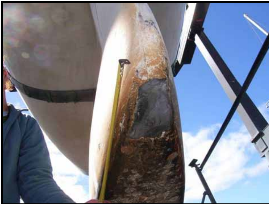
Photograph 5 (Courtesy of Hunter Marine Surveying Ltd) Damage to the lower keel.
