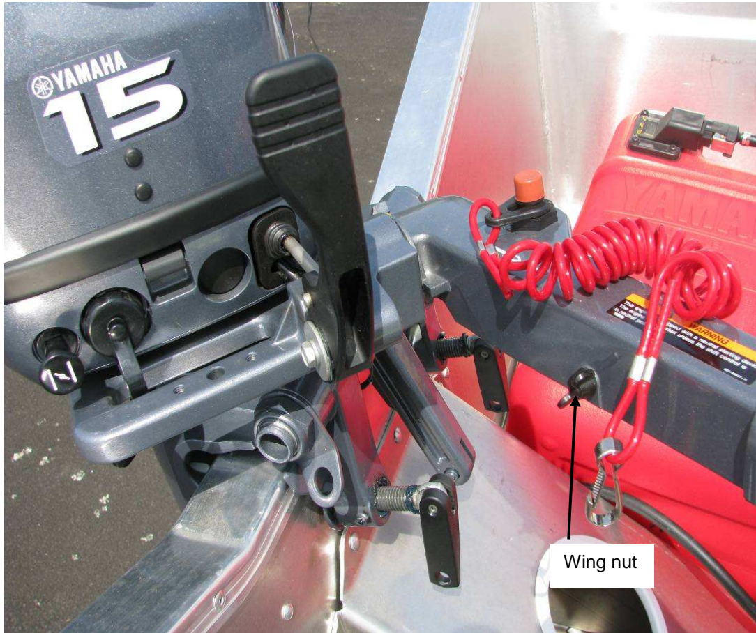
Figure 4 Similar vessel and motor showing throttle control wing nut
