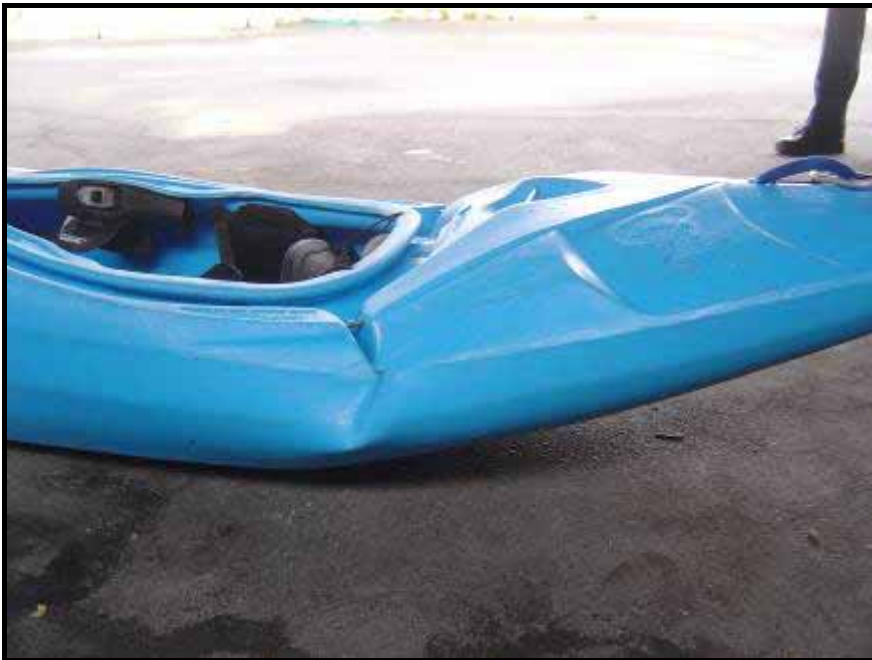
Plate 8 The fold behind the cockpit
