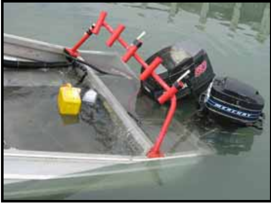
Photograph 21 Viper 1 in the stability test at 33 minutes.
