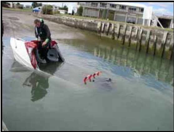
Photograph 22 Viper 1 in the stability test at 34 minutes.
