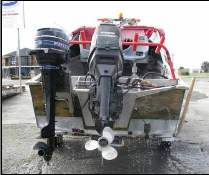
Photograph 8 The marine plywood attached to the stern.
