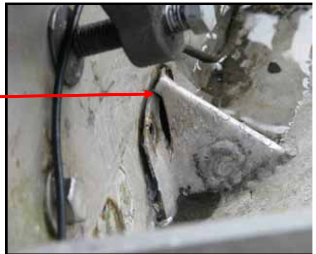
Photograph 13 A closer view of the transom-well support bracket.
