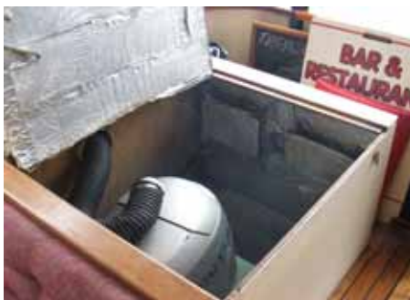
Figures 1 and 2 above show two different examples of outboards mounted inside the vessel.
