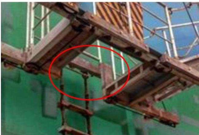
**Figure 1:** Pilot ladder/trapdoor showing the non-compliant horizontal cross-member.
