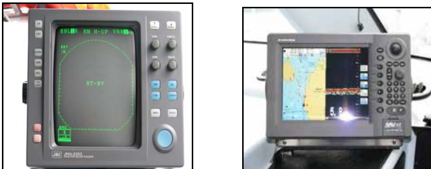
Figure 4 Radar equipment fitted on board Foveaux Express
