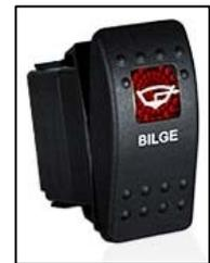
The switch should be left in the automatic position during normal operations, with the manual override only used in an emergency to by-pass the automatic function if that fails (for example, if the float switch gets jammed). It should be able to be placed in the manual 'on' position and remain there unaided should the bilge pump need to be activated manually.
