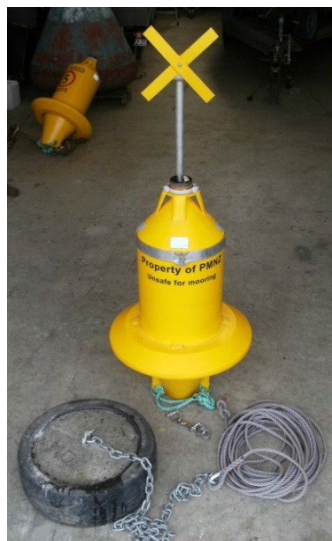
Small Special Mark (without light), topmark is an 'X' (photo Luke Grogan).
