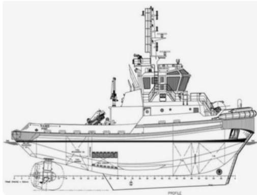
Figure 3-3: Azimuth Stern Drive Tug
